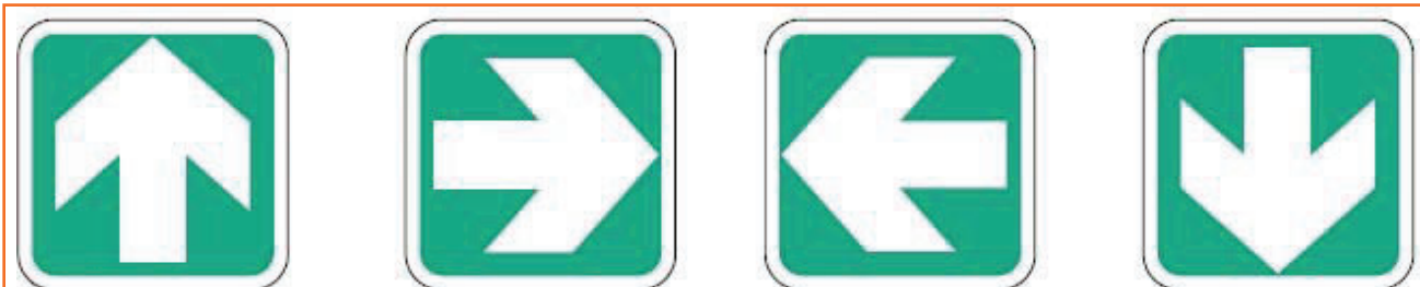
Fig.7.1.17: Signs for emergency exits
