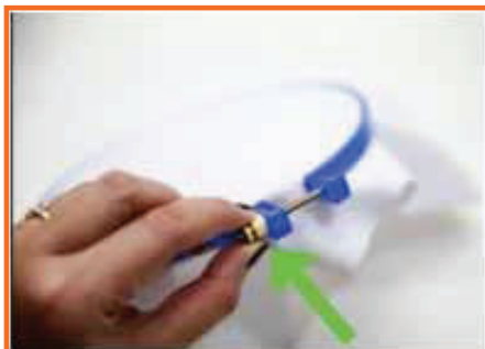
Fig.2.3.12: Metallic screw opening that can be tightened or loosened by turning the screw
